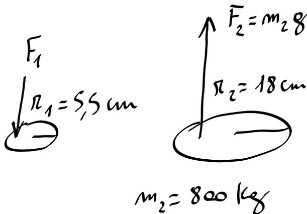
$$\frac{F_1}{S_1} = \frac{F_2}{S_2} \Rightarrow F_1 = \frac{F_2 S_1}{S_2} = \frac{(800 \text{ kg})(9,8 \frac{\text{N}}{\text{kg}}) \cdot \pi \cdot (5,5 \text{ cm})^2}{\pi \cdot (18 \text{ cm})^2}$$
