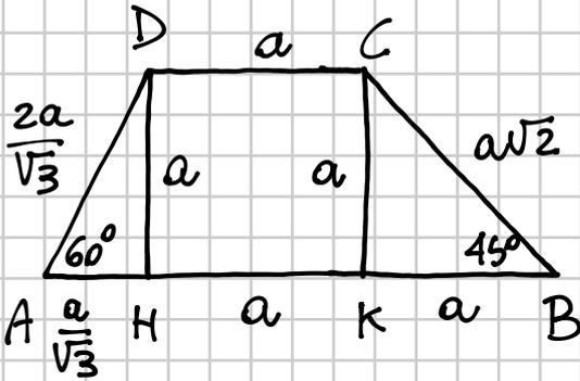
$$\overline{DH} = \overline{AD} \cdot \frac{\sqrt{3}}{2} \Rightarrow \overline{AD} = \overline{DH} \cdot \frac{2}{\sqrt{3}} = \frac{2a}{\sqrt{3}}$$
