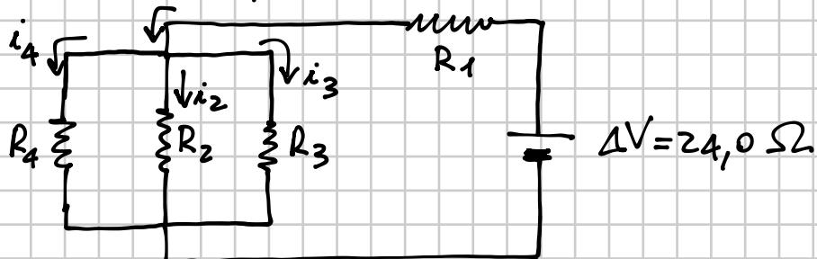
$$\frac{1}{R_{\text{eq parallelo}}} = \frac{1}{R_2} + \frac{1}{R_3} + \frac{1}{R_4} = \frac{R_3 R_4 + R_2 R_4 + R_2 R_3}{R_2 R_3 R_4}$$
