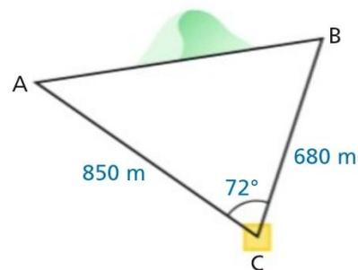
$$\overline{AB} = \sqrt{\overline{AC}^2 + \overline{CB}^2 - 2 \overline{AC} \overline{CB} \cos 72^\circ} = \sqrt{850^2 + 680^2 - 2 \cdot 850 \cdot 680 \cdot \cos 72^\circ} =$$
