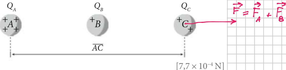
$$F = k_0 \frac{Q_A Q_C}{\overline{AC}^2} + k_0 \frac{Q_B Q_C}{\left(\frac{\overline{AC}}{2}\right)^2} = k_0 \frac{Q_A Q_C}{\overline{AC}^2} + 4k_0 \frac{Q_B Q_C}{\overline{AC}^2} =$$
