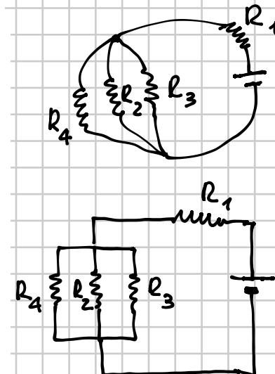
$$\frac{1}{R_{\parallel}} = \frac{1}{R_2} + \frac{1}{R_3} + \frac{1}{R_4} = \frac{1}{8,0 \Omega} + \frac{1}{12,0 \Omega} + \frac{1}{10,0 \Omega} = \frac{15 + 10 + 12}{120} \Omega^{-1}$$
