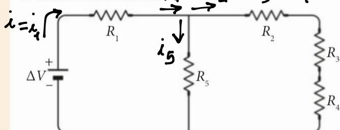
$$[R_{eq} = 100 \Omega; i = i_1 = 0,80 \text{ A}; \Delta V_1 = 64 \text{ V}; \Delta V_5 = 16 \text{ V}; i_5 = i_2 = i_3 = i_4 = 0,40 \text{ A}; \Delta V_2 = \Delta V_4 = 4,0 \text{ V}; \Delta V_3 = 8,0 \text{ V}]$$
